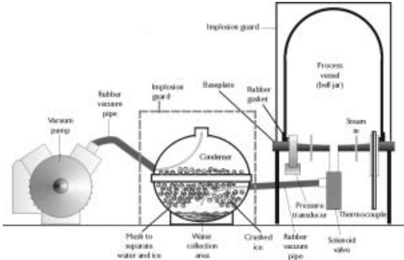
**Figure 4:** Schematic diagram of the sub-atmospheric steam decontamination apparatus. The hide samples were placed in the bell jar.
