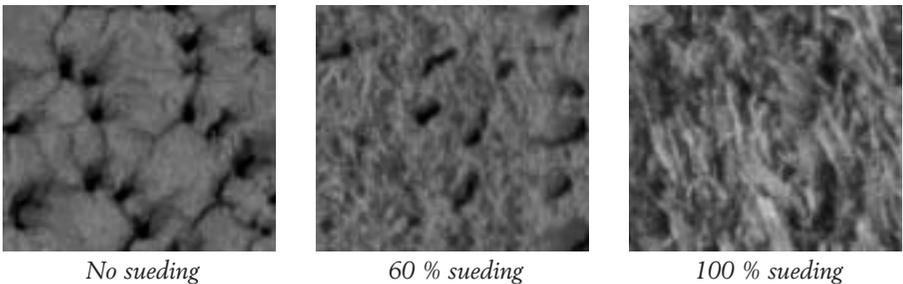
**Figure 6:** The surface of leather magnified 38 times showing no sueding, 60 % sueding and 100 % sueding.
