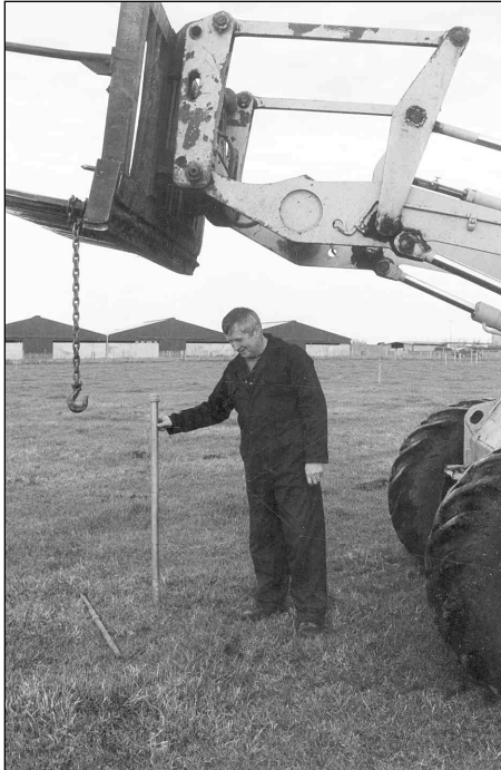
Plate 1: Soil sampler in position prior to being pushed into soil
