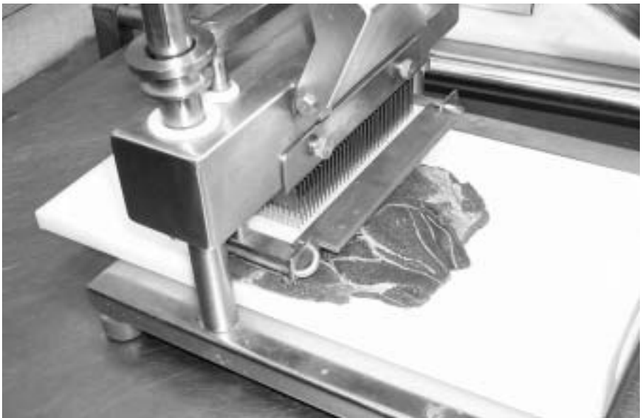
Figure 1: Tenderisation of meat sample by 36 blade manually operated tenderiser.
