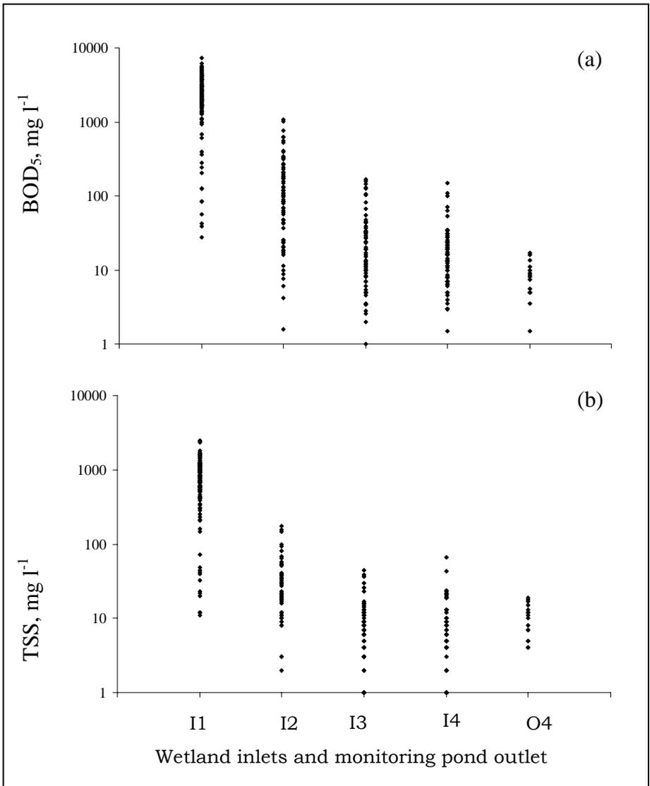
**Figure 5:** Log reduction of (a) five day biological demand (BOD<sub>5</sub>) and (b) total suspended solids (TSS) between wetland inlets (I1-I3) and inlet and outlet of final monitoring pond, respectively (I4-O4) during the monitoring (April 2001 – September 2003).
