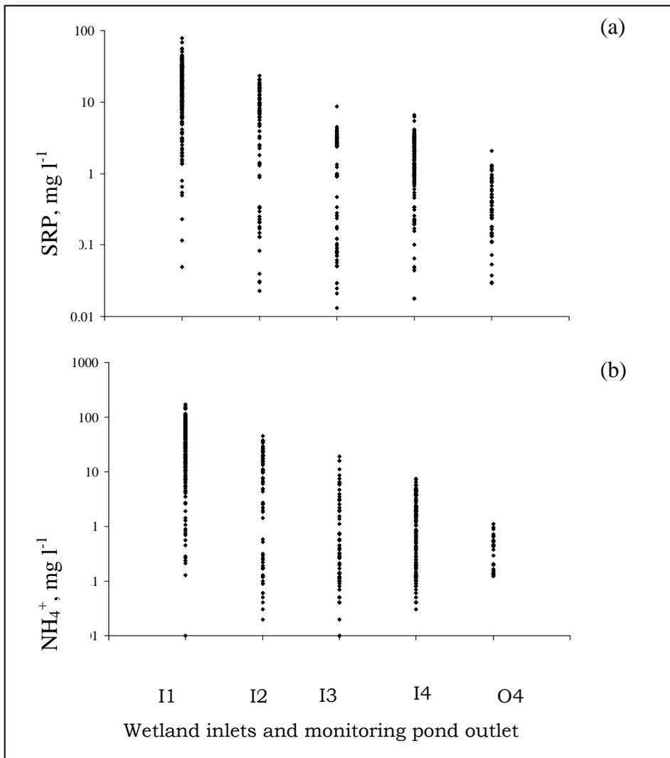
**Figure 4:** Log reduction of (a) soluble reactive phosphorus (SRP) and (b) ammonium ( $\text{NH}_4^+$ ) in  $\text{mg l}^{-1}$  between wetland inlets (I1-I3) and inlet and outlet of final monitoring pond, respectively (I4-O4) during the monitoring period (April 2001 - September 2003).
