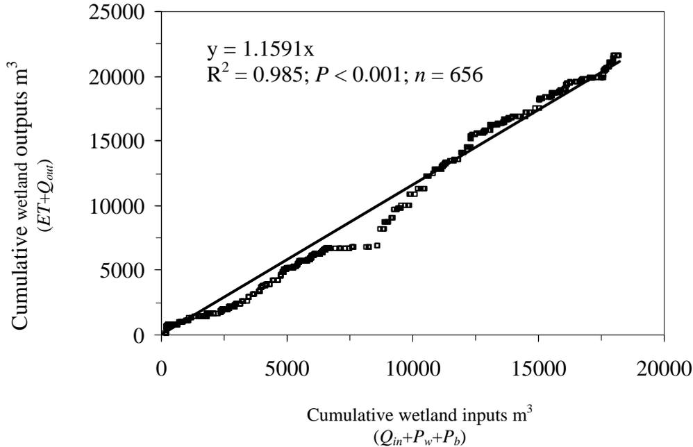
**Figure 3:** Relationship between cumulative wetlands inputs (farmyard dirty water in ( $Q_{in}$ ), precipitation on wetland surface area ( $P_w$ ), and inflow from precipitation on surrounding wetland banks ( $P_b$ )) and cumulative wetland outputs (evapotranspiration from the wetland surface area ( $ET$ ), and wetland surface outflows ( $Q_{out}$ )).
