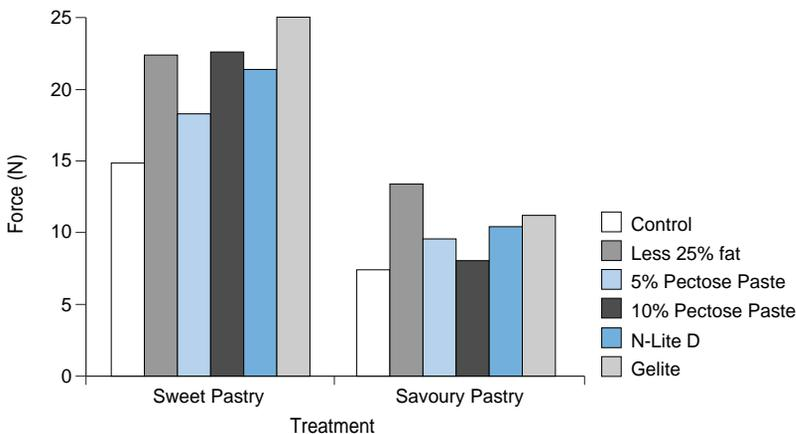
**Figure 10:** Effect of N-Lite D, Pectose Paste or Gelite on texture of reduced fat (-25%) sweet and savoury pastry.
