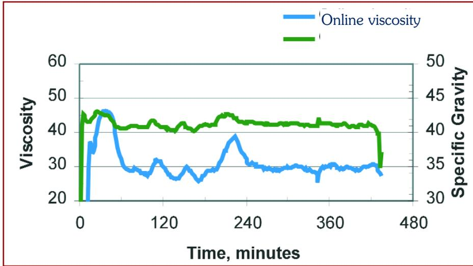
Fig. 2. Trend showing viscosity and specific gravity measured on-line during manufacture of whole-milk powder. Viscosity was measured using a vibrating rod in torsional mode. Specific gravity was measured using vibrating U-tube densitometer.
