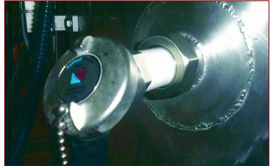
*Fig. 5. Fibre optic probe installed in cheese vat.*
