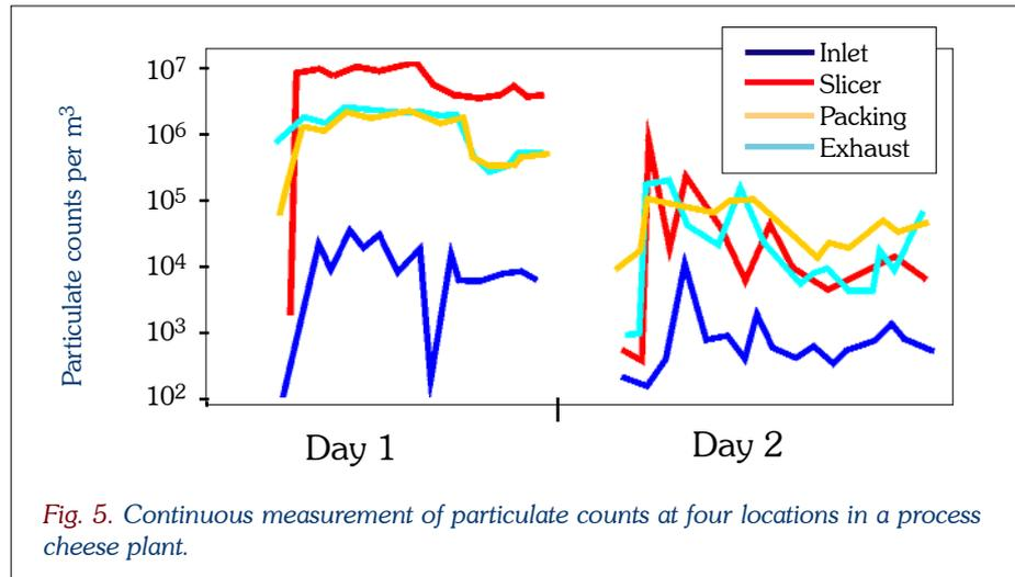
*Fig. 5. Continuous measurement of particulate counts at four locations in a process cheese plant.*
