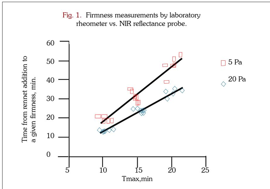
study the sensors were able to predict cutting time with an average deviation of 1.5 minutes, with good repeatability for replicates at the same conditions. This was achieved without having to incorporate any process conditions into the analysis. A 10% increase in rennet concentration was found to reduce the set-to-cut time by about 2 minutes, and this was equivalent to increasing the setting temperature by 1 degree Celcius . All three sensors detected these changes equally well.
