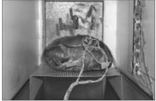
Figure 4: Flash roasted ham in vacuum cooler chamber with thermocouples inserted at various points of the ham.
