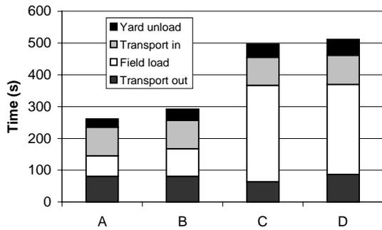
**Fig. 1. Bale transport, time per cycle.**
