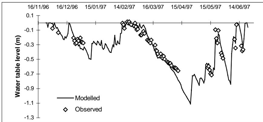
**Fig. 5:** Water table level from the WT model compared to observed values at pipe D2, Cowlands
