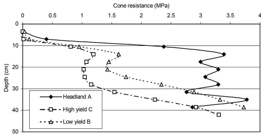
**Fig. 12:** Penetrometer readings in high- and low-yielding areas, Cappoquin, 1999
