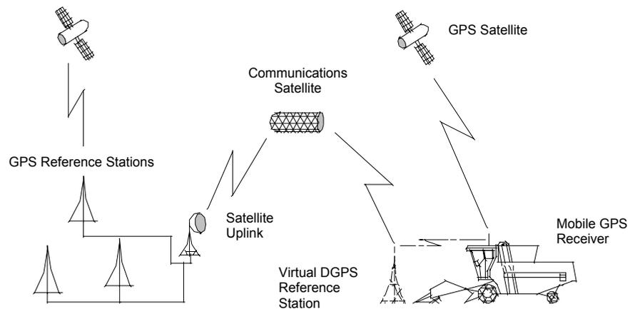
**Fig. 2:** Schematic of 1998 yield mapping system using communications satellite for reference signal
