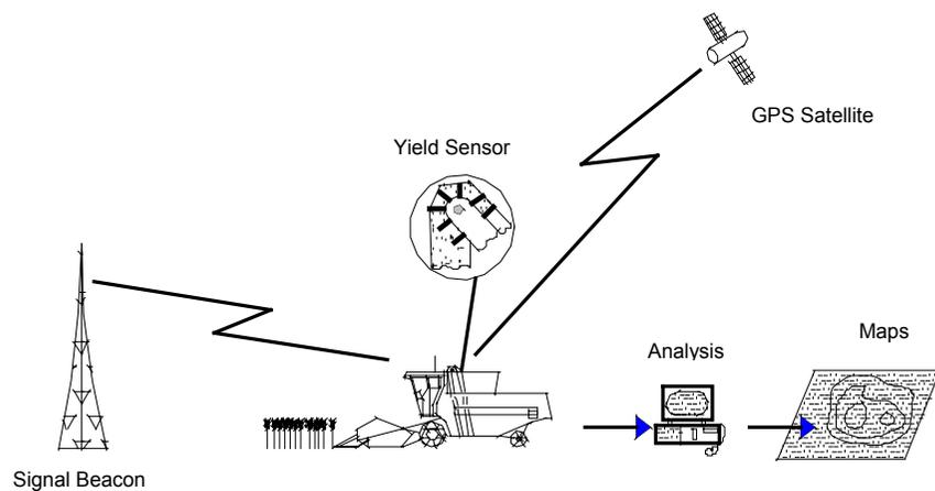
**Fig. 1:** Schematic of a yield mapping system
