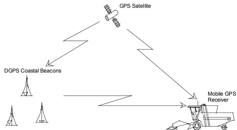
**Fig. 3:** Schematic of 1998 yield mapping system using coastguard beacon for reference signal
