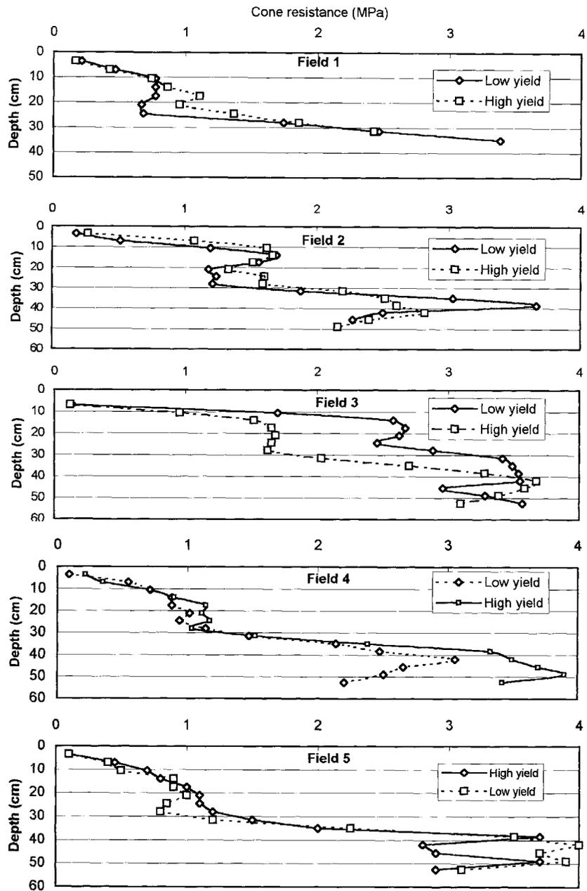
Fig. 10: Results of soil compaction tests in five yield-mapped fields, Carlow, 1999
