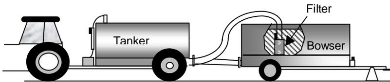
**Fig. 2:** Set-up for the filter trials with obstacles
