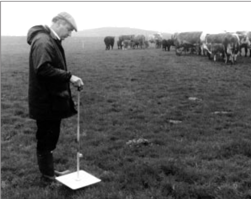
A plate meter can be used as a useful grassland management aid
