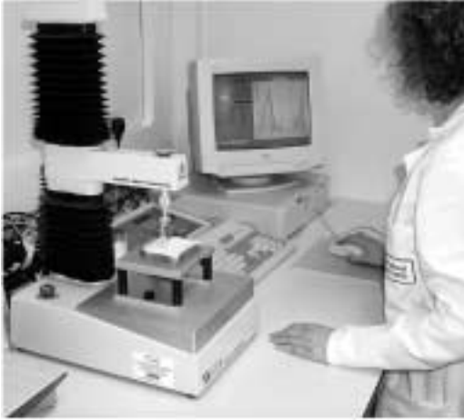
Figure 3: The texture analyser (TAXT2i) is used to assess characteristics such as the hardness, springiness and staling rate of bread crust and crumb.
