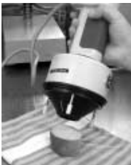
Figure 3: The Minolta Chroma Meter measures colour in numerical terms.
