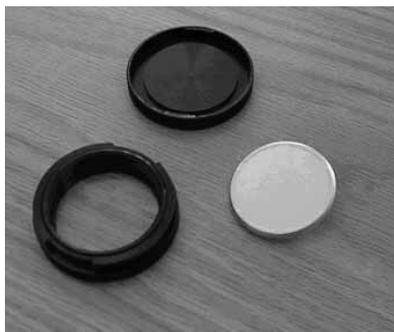
**Figure 1.** Near infrared spectrophotometer and camlock transreflectance sample cell.
