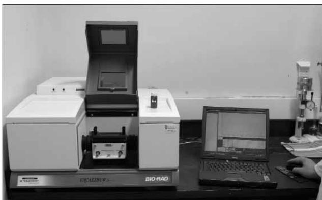
**Figure 7.** Mid-infrared spectrophotometer with attenuated total reflectance sample cell.
