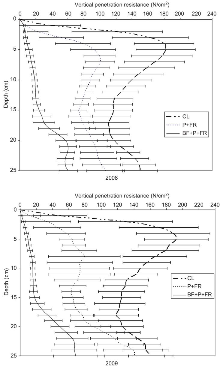
Figure 6. Vertical penetration resistance at depths between 0 and 25 cm according to three different planting and ridge formation methods during 2008 and 2009.
