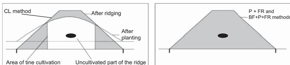
Figure 3. Cross-sectional area of loose soil in the ridge according to the CL, P+FR and BF + P + FR methods.
