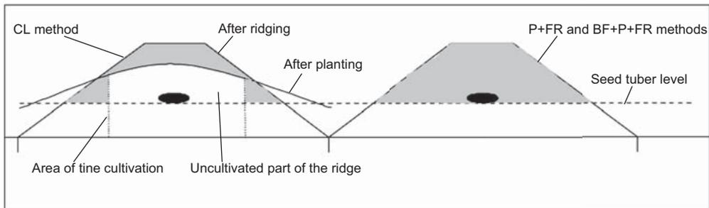
Figure 4. Net cross-sectional area of loose soil in the ridge according to the CL, P+FR and BF+P+FR methods.
