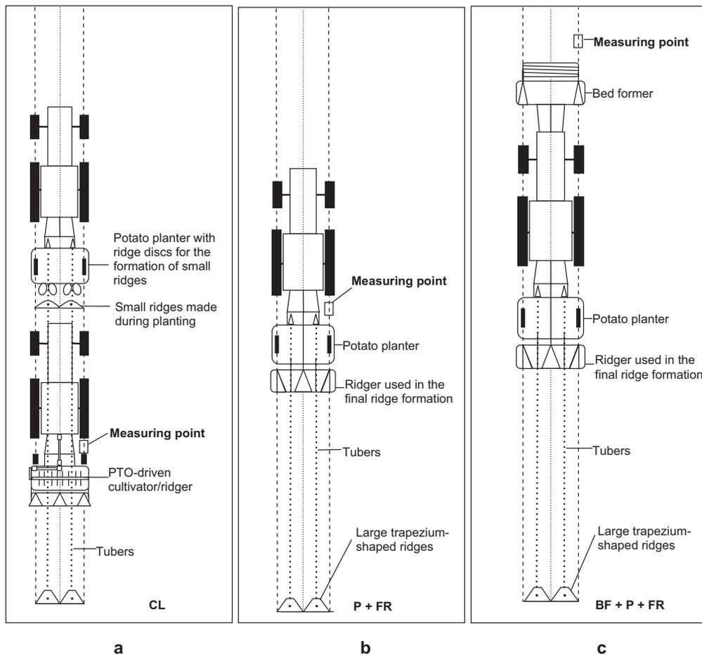
Figure 2. Diagram of planting and ridge formation according to the CL (a), P+FR (b) and BF+P+FR (c) methods with the relevant measuring points.
