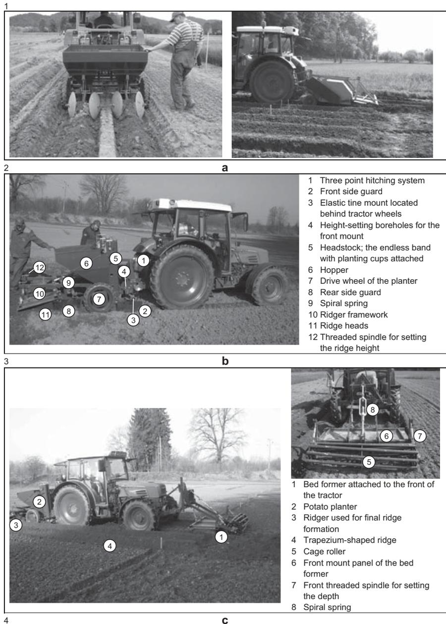
Figure 1. (a) the CL method consisted of a potato planter with a ridger for the formation of small ridges and a PTO-driven cultivator/ridger to be used before potato emergence; (b) the P+FR method consisted of a potato planter with a ridger for final ridge formation; (c) the BF+P+FR method: potato planter with a ridger for final ridge formation, and a special bed former attached to the front of the tractor pushing the loose soil for ridge formation off the wheels of the tractor.
