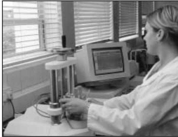
▲ Measuring the elasticity modulus of glutenin using a Bohlin VOR rheometer
