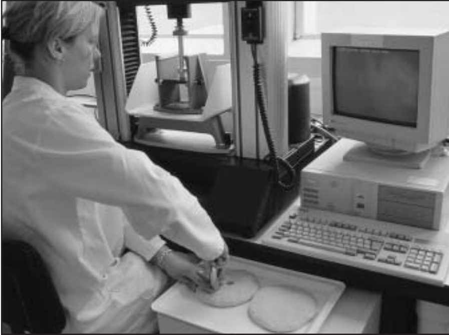
▲ Measuring pizza bases for texture profile using an Instron universal testing machine
