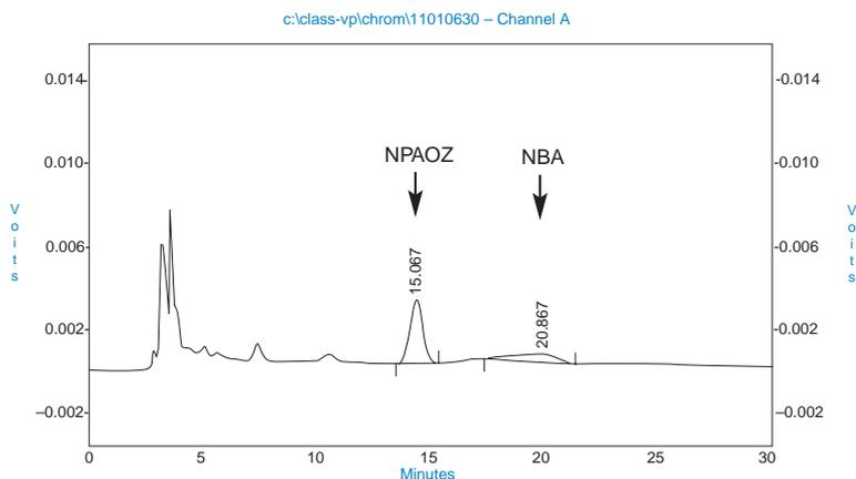
**Figure 3 (b).** Chromatogram of tissue extract containing NPAOZ after Oasis™ MAX plus Oasis™ HLB clean-up
