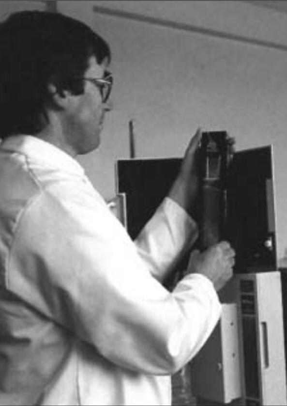
**Figure 3.** Collecting near infrared spectra of meat samples for confirmation of freshness
