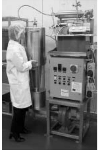
*Using fluidised bed technology to encapsulate vitamin C. ▶*
