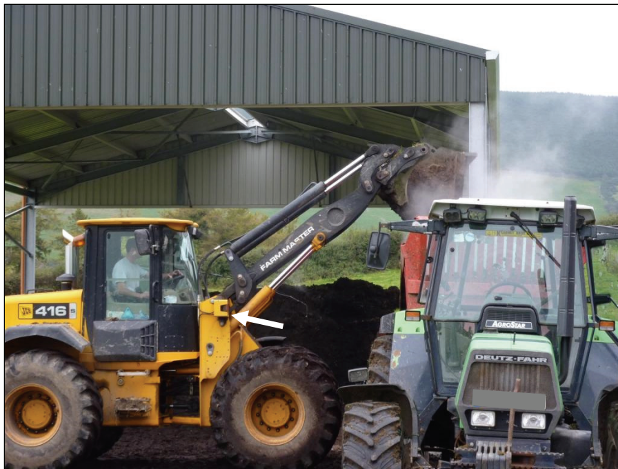
Figure 1. SMC is tipped into a spreader by the front-end loader at indoor site 4. Stored SMC is visible in the background. The white arrow indicates where the monitor was attached to the outside of the loader.
