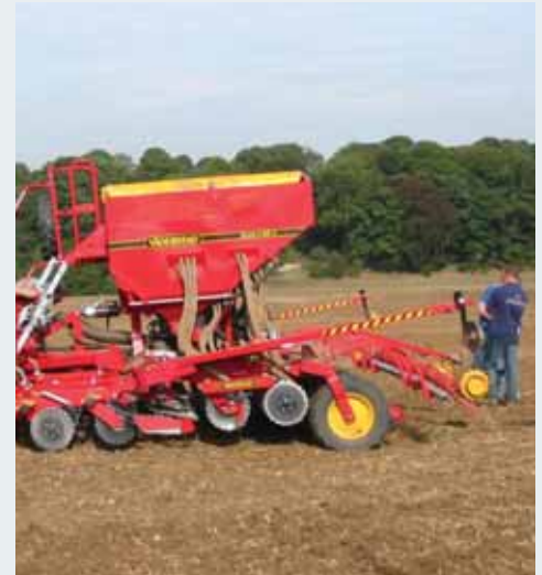
Seeder suitable for sowing into minimum-till ground.
