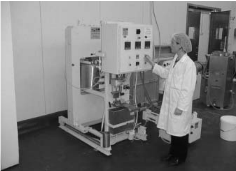
High hydrostatic pressure processing unit (EPSI, Belgium)
